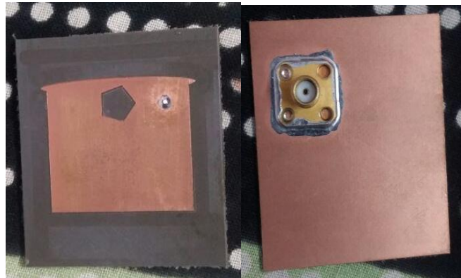
Fig.3. Fabricated Rectangular patch with Elliptical edge and pentagon. (a) Front view, (b) bottom view
