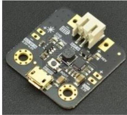
Fig.3. Energy harvesting module (SPV1050)
