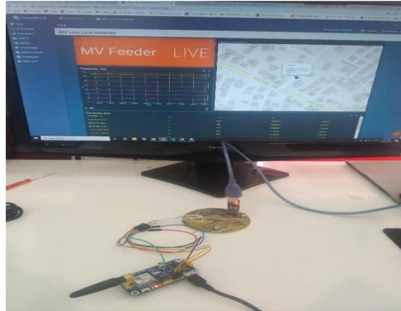
Fig.11. IoT server front end indicates sensor data
